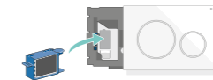
ACCESSIBLE The ceramic honeycomb filter can be easily accessed via the actuator plate.
